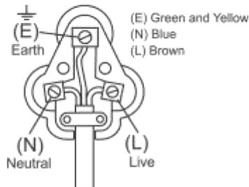
**If your appliance has only two wires (Blue, Brown) then it does not need to be earthed. Connect a three pin plug as shown below**
