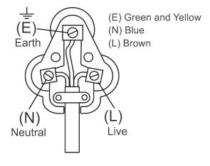
If your appliance has only two wires (Blue, Brown) then it does not need to be earthed. Connect a three pin plug as shown below
