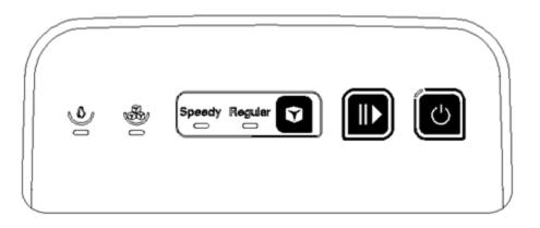
The indicator light for POWER will flash after ice machine has been plugged in, press POWER and the machine will enter standby mode. During operation, pressing this button will return machine to standby mode
