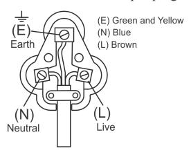
If your appliance has only two wires (Blue, Brown) then it does not need to be earthed. Connect a three pin plug as shown below
