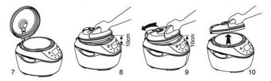
\*In the process of turning the lid, please ensure that the height between the lid and the upper edge of the cooker is always 10cm. This is to smoothen the turning and removing process.
