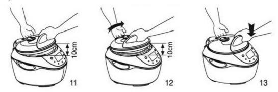
\*In the process of turning the Lid, please ensure that the height between the Lid (2) and the upper edge of the cooker is always 10cm. This is to smoothen the turning and removing process.
