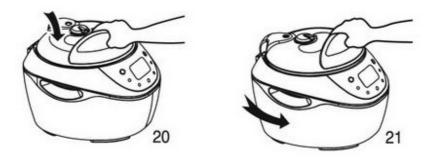
5. Before you begin cooking adjust the pressure limiting valve to "Airtight" (airproof) position. You will notice that the floating valve is dropped, as the pressure inside the cooker increases, the floating valve rises. The floating valve sinks again when the heating process is over and once you have released the pressure inside by turning the pressure limiting valve to an "Exhaust" position. (Figure 22-a & 22-b).
