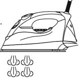
Note: It may be necessary to press the burst of steam button a few times to start this function.
